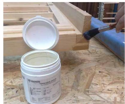
Teknoseal 4000 applied by brush to exposed end grain prior to factory finishing
