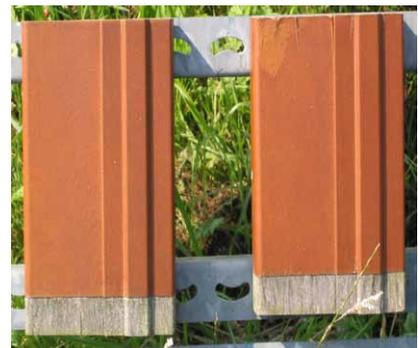
After 24 months exposure, moisture ingress on the untreated end grain on the right hand component has caused splitting, discolouration and adhesion failure at the cut edge
